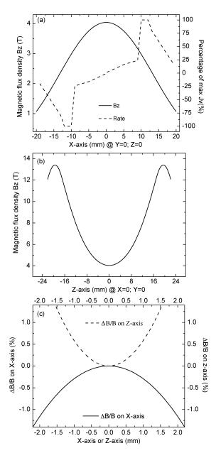
Fig. 3. Magnetic profile of the designed double bulk HTS disks. (a) *B*-field in the transverse direction and the distribution of applied percentage of  $J_v$ . (b) *B*-field on the transverse axis in the central plane of two bulks; two maxima of field strength at  $\pm 19.5$  mm. (c) Distribution of the region of uniformity field.
