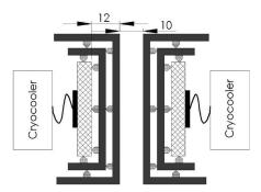
Fig. 4. Schematic concept of the pair of HTS bulk disks and the cooling method; the unit is mm.
