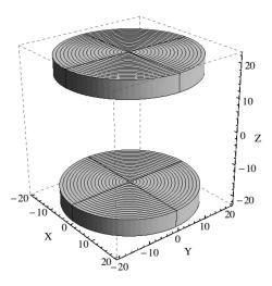
Fig. 1. A pair of HTS bulk disks constructed from two thin cylindrical bulk HTS simulated with Radia code. The concentric circles signify that the cylinder is made with multi-layer current rings; the unit is mm.
