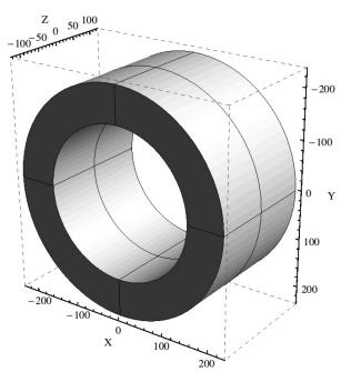
Fig. 5. The diagram and dimension of the solenoid coil of magnetization magnet system. The unit is mm.
