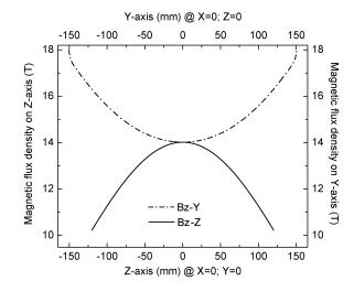
Fig. 6. Profile of the distribution of the magnetic field on the axis of the solenoid of the magnetization system.
